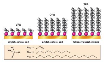
Figure 1. Various organophosphonates were measured using MP-SPR.
