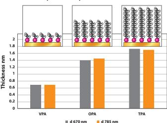
Figure 4. SAM thicknesses: vinylphosphonic (VPA), octylphosphonic (OPA), and tetradecylphosphonic acid (TPA).
